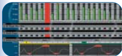
MCS 4000 Remote control and remote monitoring software. The MCS 4000 displays all status readouts of a complete multichannel system on a single screen. The integrated spectrum analyzer and frequency management software can be updated through the Internet. MCS 4000 scans the UHF band, automatically calculates the optimum frequencies, and programs them into the receivers while you have a cup of coffee!
